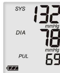
LED display: This large display shows data from measurements in self-measurement mode. You can easily check the time until the next ABPM measurement in addition to values in self-measurement mode. There are also icons for battery level, Bluetooth status, AFib<sup>2</sup> detection, clock, mode and memory status.
