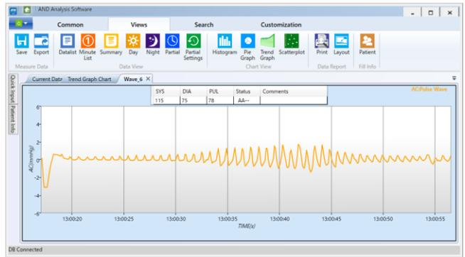
Both the TM-2440 and TM-2441 record blood pressure as an oscillometric waveform. With our new analysis software you can check the waveform record for each measurement. Quickly determine the accuracy of measured values.
